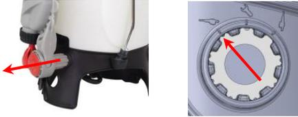
Pull the pump lever out at the pump-lever joint to the first catch (adjustment position). Turn the pump lever to the desired position and slide it back in again until it's completely locked into position.
